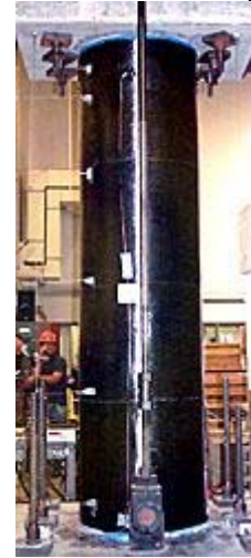
Photo: 3 Completed Laying with Build Seal Prepreg
